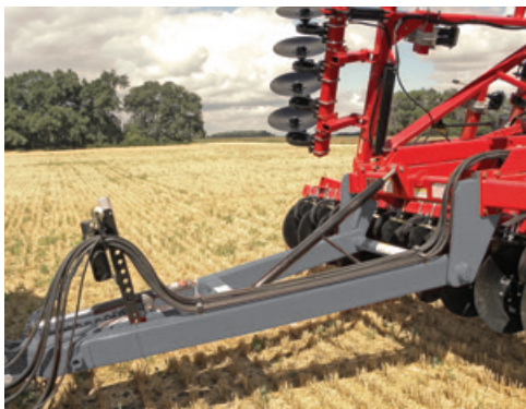
Rigid hitch keeps the front and rear of the 657 DCR level.
