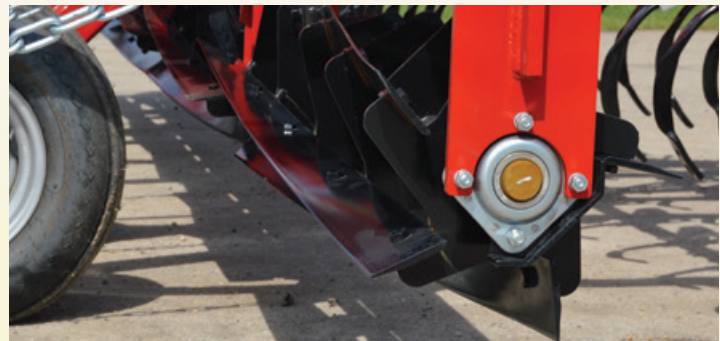
The cutting reel pulverizes the ground to mix soil and incorporate chemical accurately at the required depth. This balanced and heavy cutter has self-aligning bearings.
