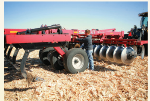
Heavy-duty 4 x 8-inch (10 x 20 cm) frame adds additional weight to keep the tool in the ground and ripping through even the heaviest residue.
