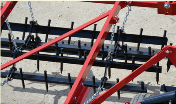
The spike harrow drags the soil and breaks up clods to smooth the ground.
