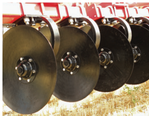
Concave discs utilize a 6-bolt hub and are 22 inches (56 cm) in diameter – allowing for a maximum working depth of 5 inches (13 cm).
