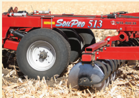
385/65R 22.5 used truck tires are standard on walking beam axles.
