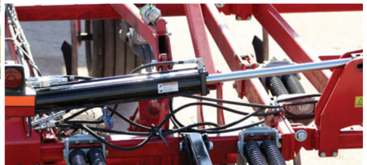
Hydraulics on the Wil-Rich 2500 Series Chisel Plow are a 10-inch (25.4 cm) stroke Prince wing fold cylinder that varies the bore size to accommodate lift circuit phasing.
