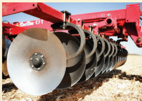
Individually mounted C-spring, 28-inch (71 cm) disc blades provide a split-the-middle tillage advantage.
