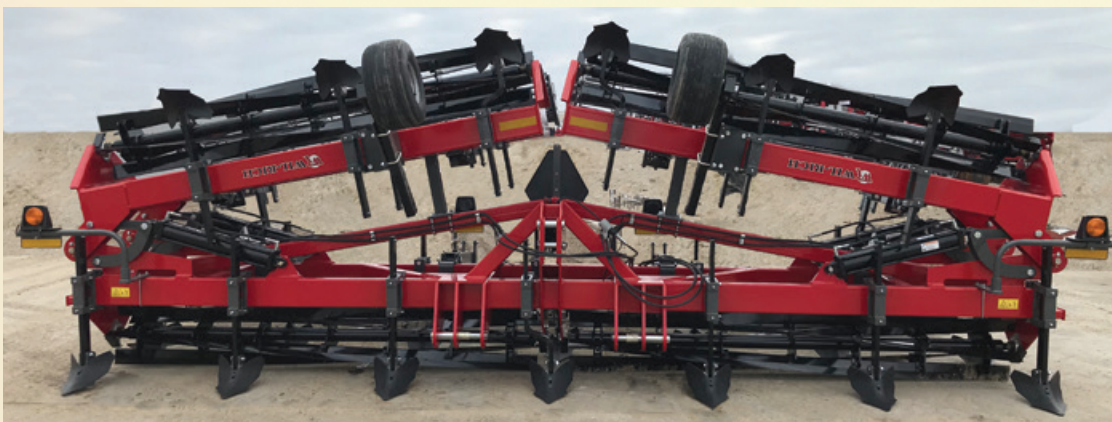
Above: The Wil-Rich 1500 Series Bedder Finisher has four wing fold cylinders and folds to 20'5" ft for easy transport.
