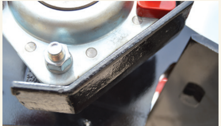
Bearing guard protects bearing from debris.
