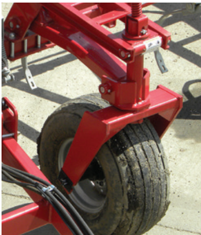
Hydraulic front casting wheels on the main frame of the QX 2 are equipped with a wheel damper kit for stable transport assistance.
