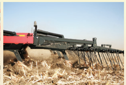
Two ranks of shanks are 55 inches (145 cm) apart; the closest shanks are 48 inches (122 cm) apart on the rank, promoting excellent crop residue flow.
