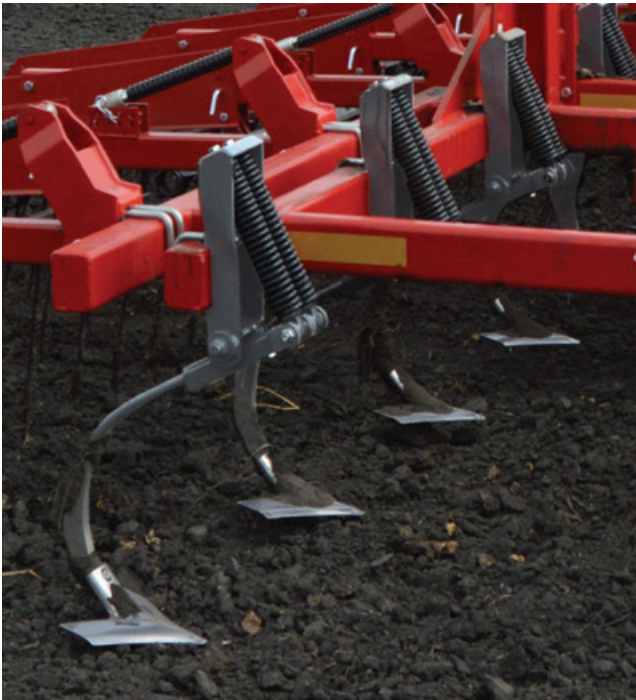
Single spring and twin spring options with 7-inch spacing are available on the XL 2 and QX 2 .
