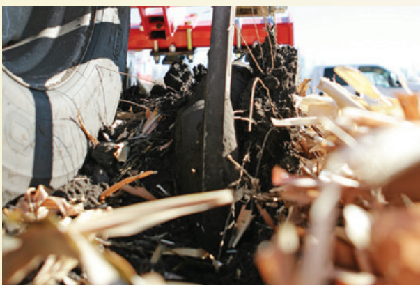
The 4-inch (10 cm) concave twisted shovels are designed to more efficiently bury and mix crop residue.
