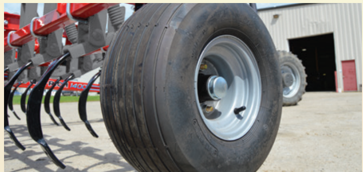
Gauge wheels control the depth of the Wil-Rich 1400 Seedbed Finisher in rolling ground.
