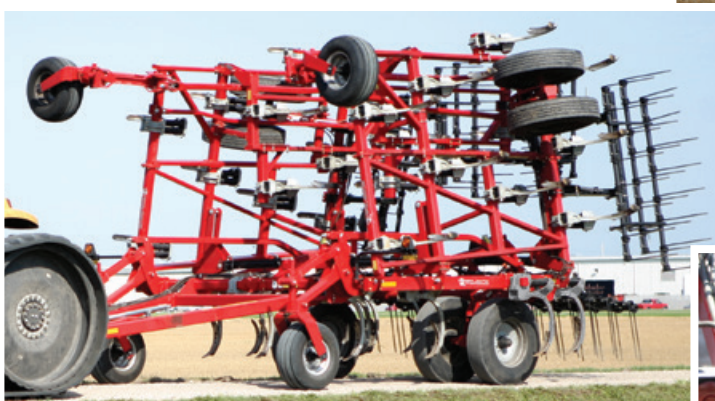
The 2500 Series Chisel Plow folds to a compact transport package to easily move to the next field.
