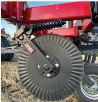
Optional 20-inch (51 cm) spring-loaded coulters easily slice through some of the heaviest residue.
