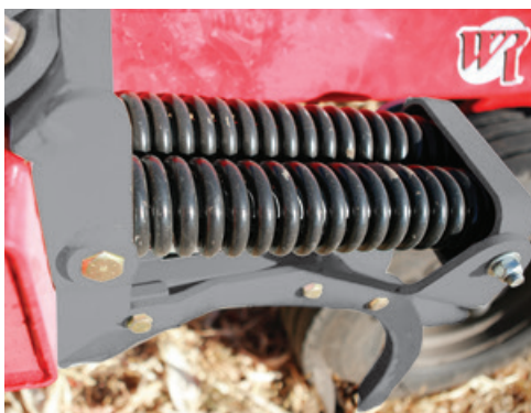
Heavy-duty, 1,400-pound (635 kg) spring cushion trips stay true in the toughest soils.
