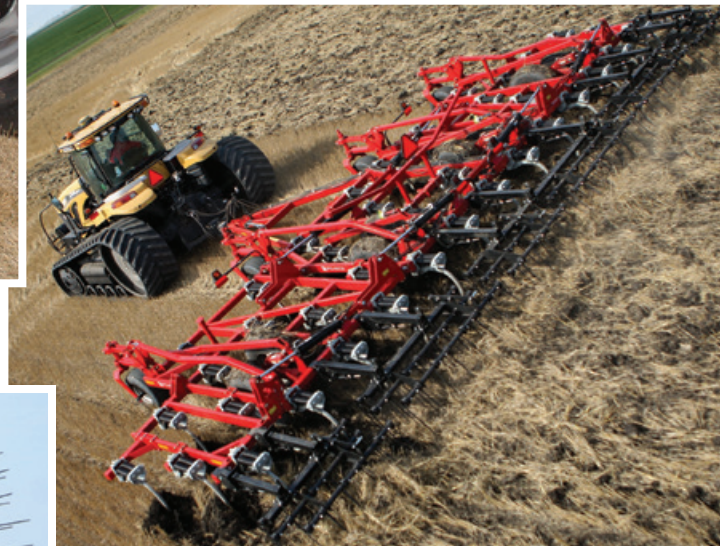
The deep frame is 140 inches (356 cm) front to back, providing superior trash flow for today's higher residue crops.
