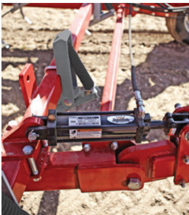
A weight transfer kit is available for the QX 2 and is standard on units with 5- and 6-foot (1.5 and 1.8 m) outer wings, as well as 5-section units. The kit is optional on all other models. This kit puts weight on the floating hitch and the front gauge wheels to create more stability during transport.
