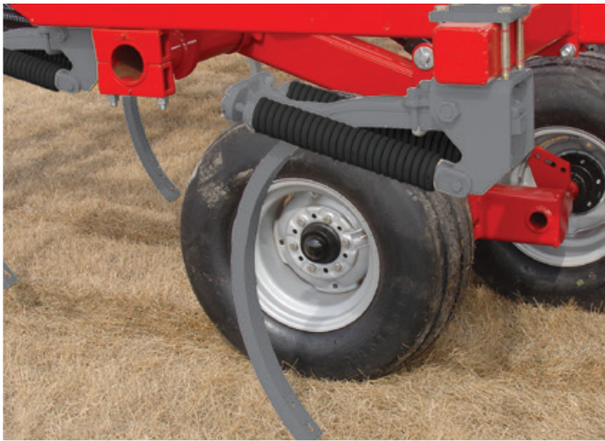
The 650 lbs. (295 kg) extension spring trip assemblies of the 2500 series Chisel Plow are built to tackle the toughest soils.
