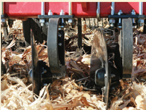
Coulters are indexed to shanks for a 7½-inch (19 cm) working pattern.
