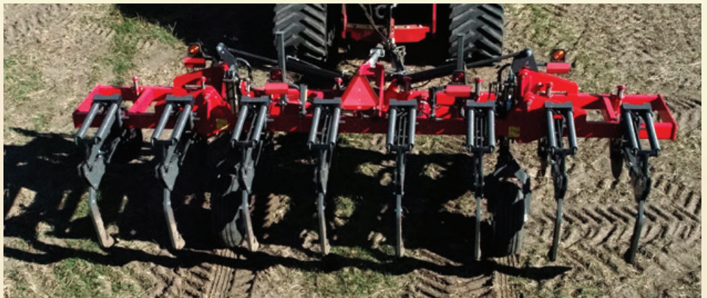
Massive 3,500 lb. (1.6 MT) twin spring reset trip assembly keeps shanks in the ground.
