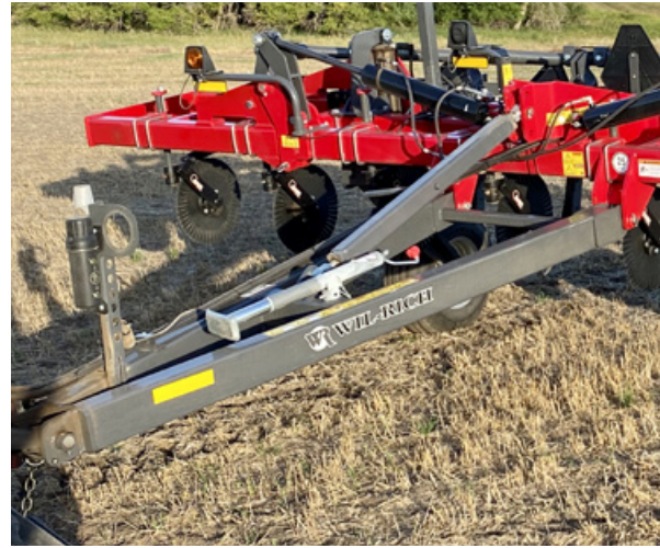
Pull type hitch with hinged tongue is optional. Frames are 3-point adaptable for Cat II or Cat III.
