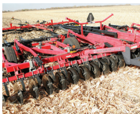
Frame strength and ballast are supported by large, 6 x 4 inch (15 x 10 cm) main frame.
