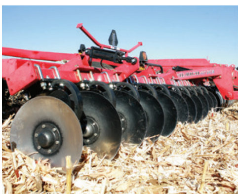
Front coulters can be hydraulically raised and lowered for varying residue conditions.
