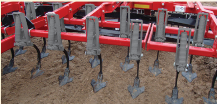
Shanks on the Wil-Rich 1400 Seedbed Finisher penetrate the ground to break up the soil. The shank works well on flat ground.
